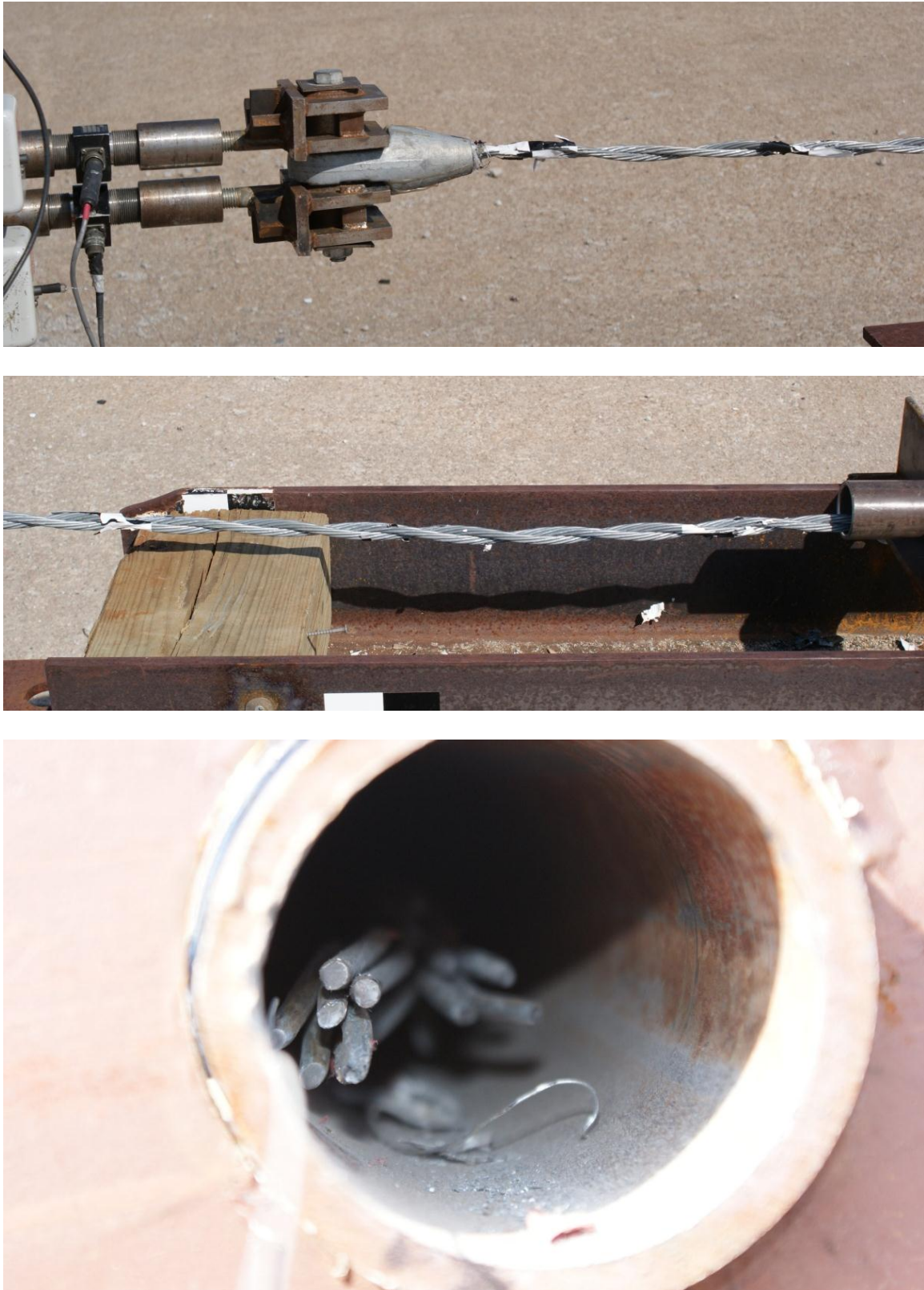
Figure 57. Upstream Wire Rope Damage, Test No. DTC-1
