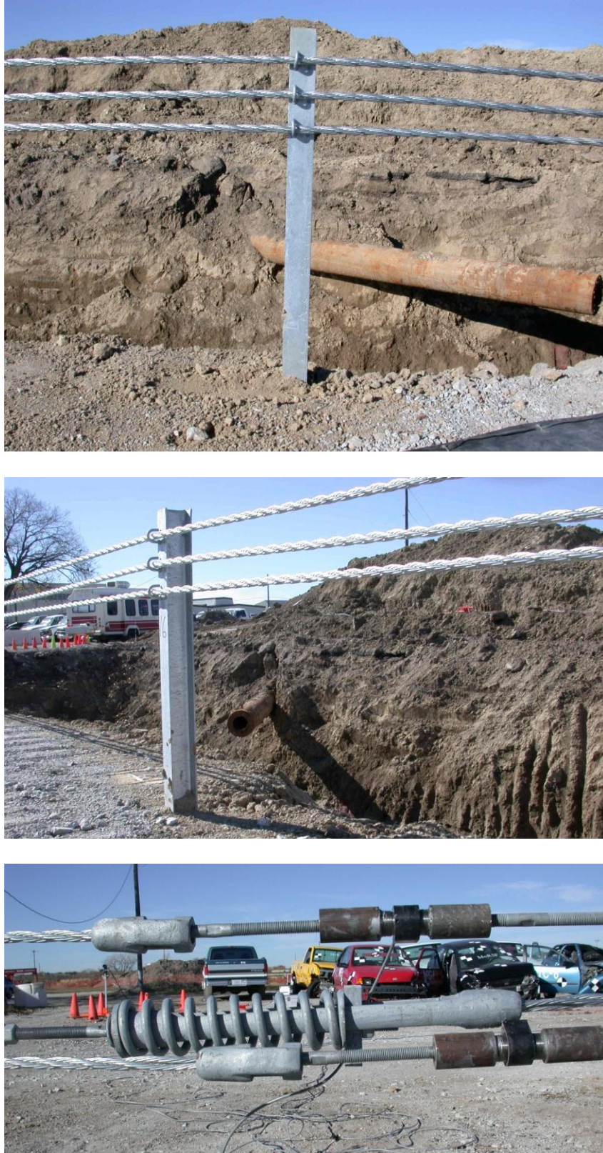
Figure 201. Line Posts and Cable Compensator, Test No. CS-1
