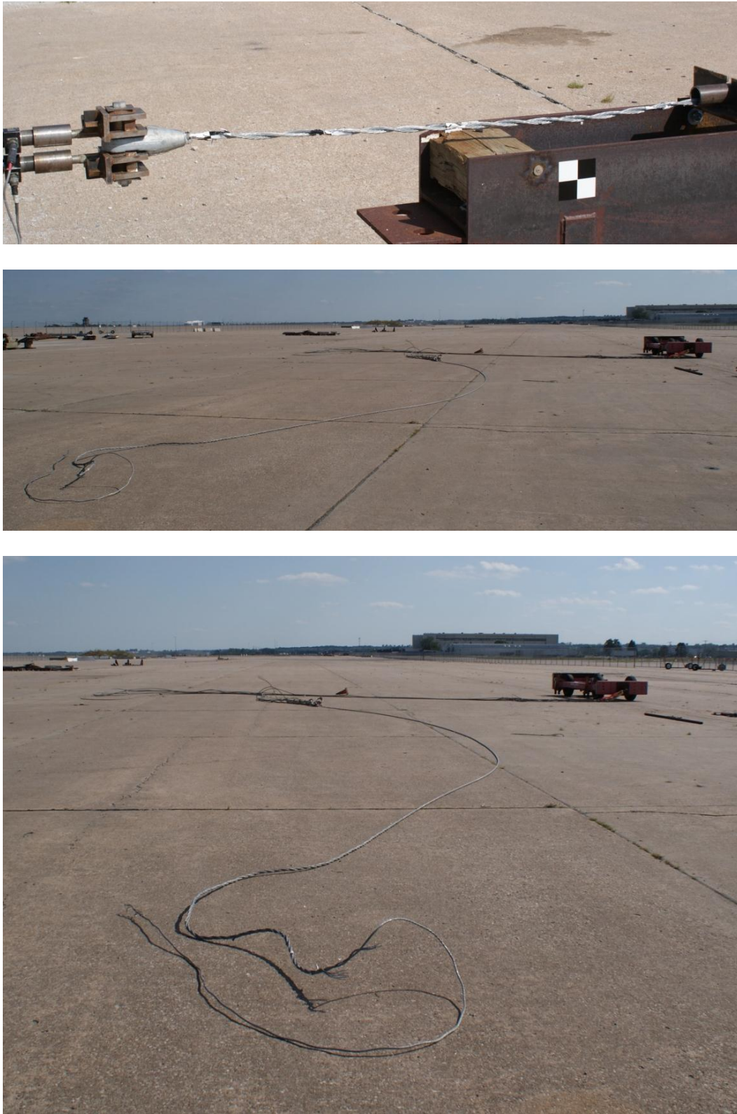
Figure 55. Bogie and Wire Rope Final Position, Test No. DTC-1
