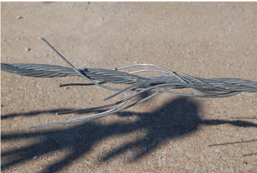
Figure 134. Wire Rope Damage, Test No. DBC-4
