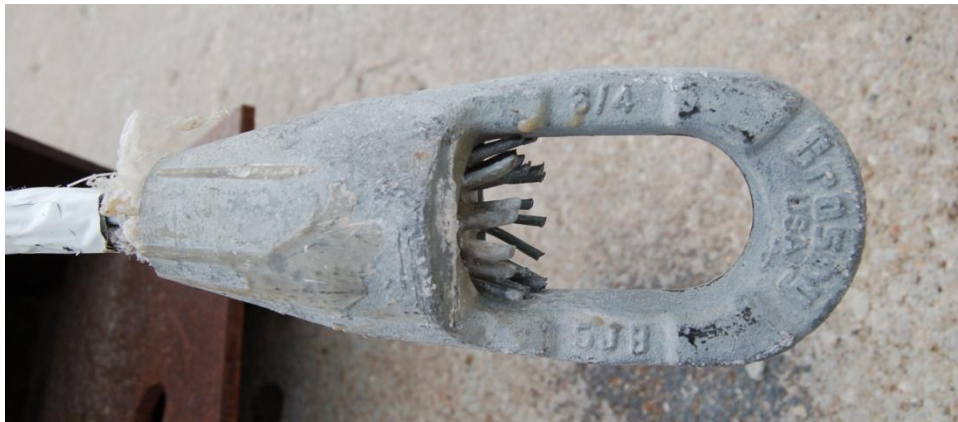
Figure 73. Upstream Wire Rope Socket, Test No. DTC-3
