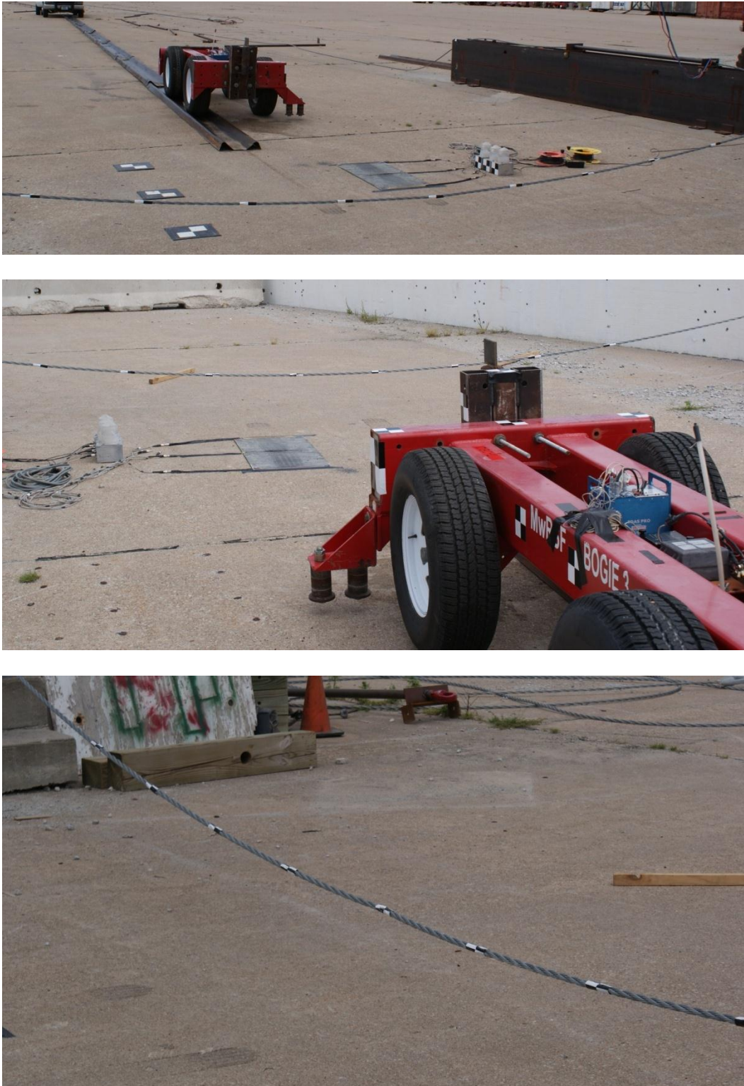
Figure 115. Final Position of Wire Rope and Bogie Vehicle, Test No. DBC-1
