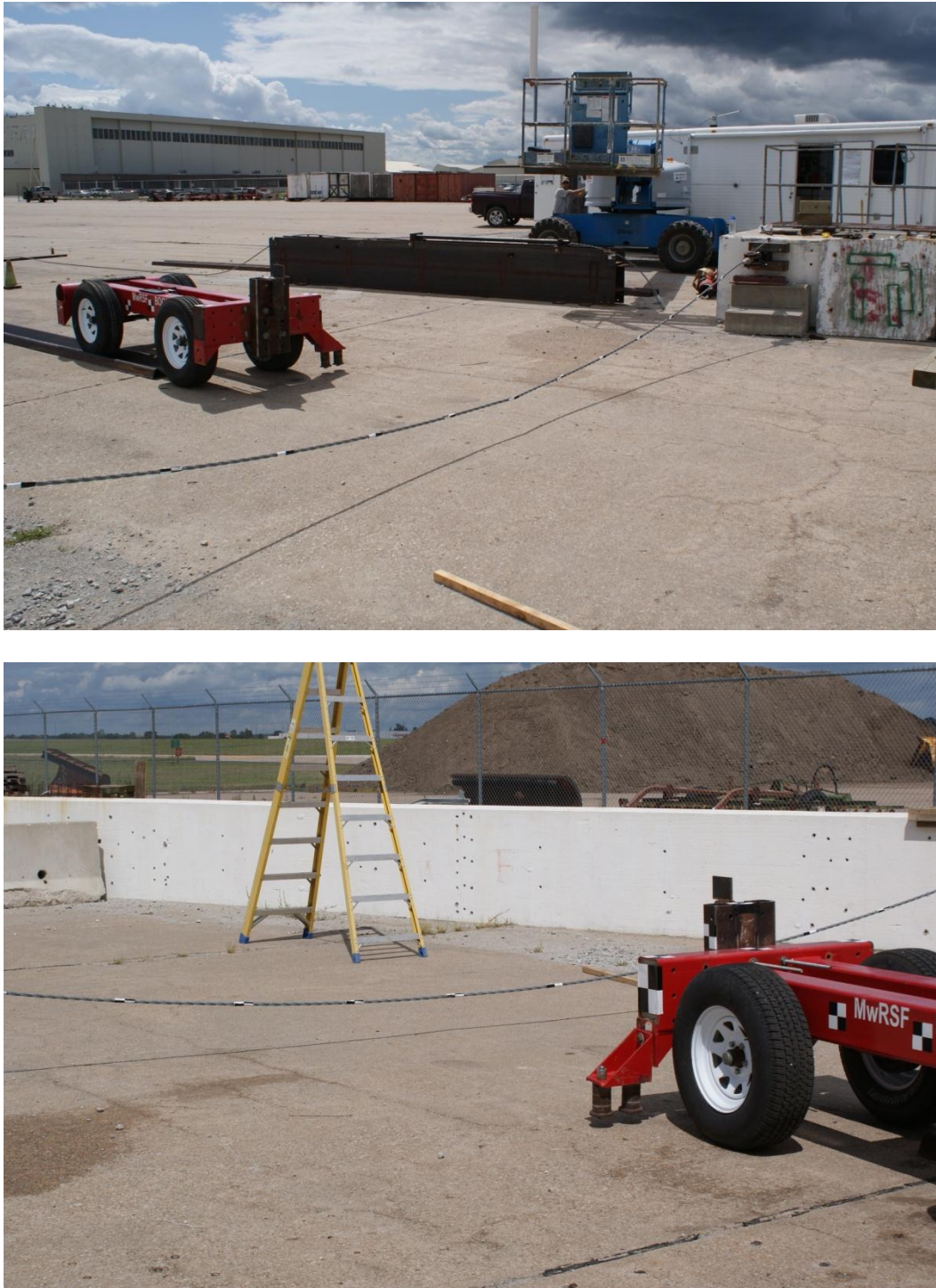
Figure 116. Final Position of Wire Rope and Bogie Vehicle, Test No. DBC-2
