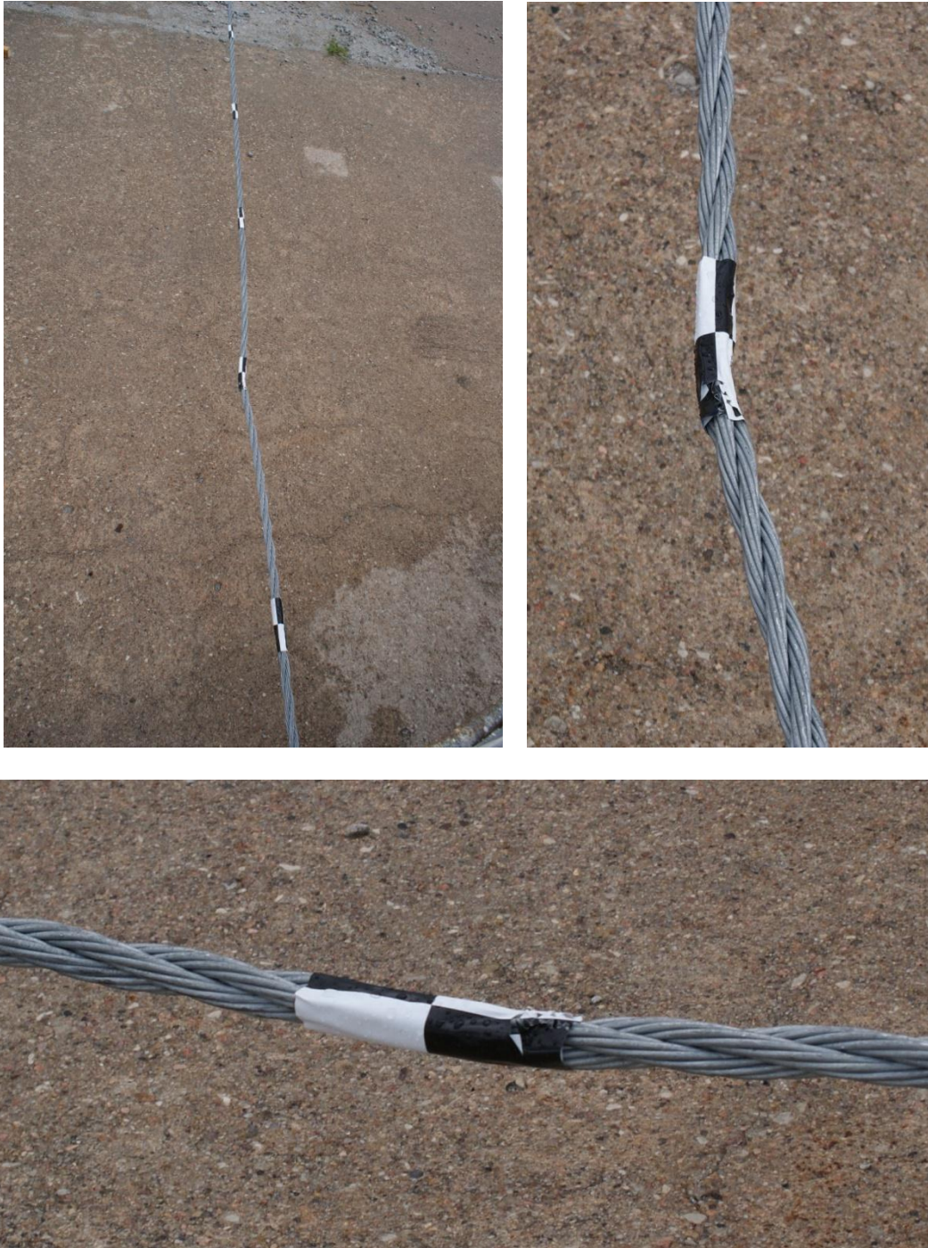
Figure 118. Wire Rope Damage, Test No. DBC-2
