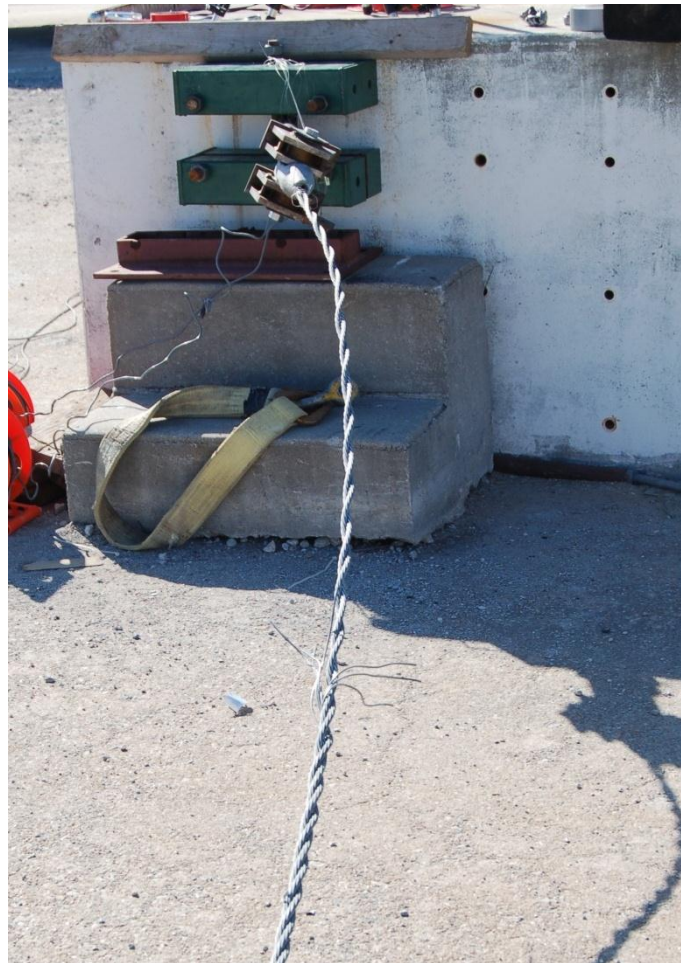
Figure 132. Wire Rope Damage, Test No. DBC-4
