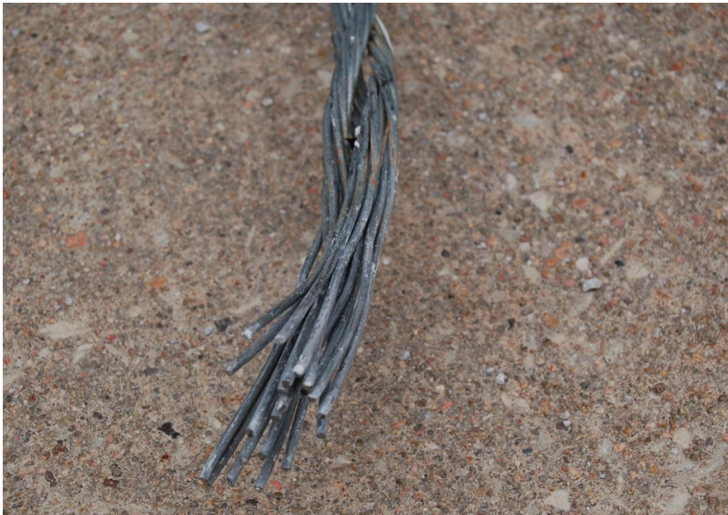
Figure 68. Downstream Wire Rope Pullout, Test No. DTC-2
