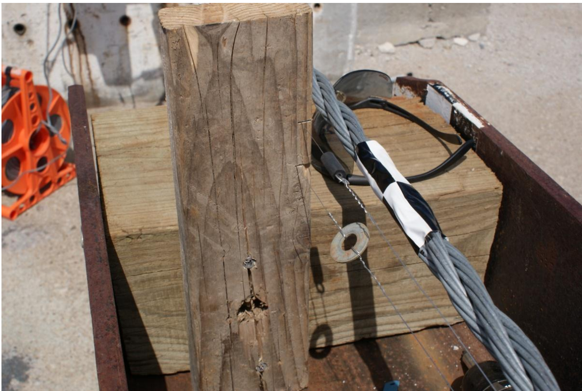
Figure 53. String Potentiometer Alignment and Configuration Details, Test No. DTC-1
