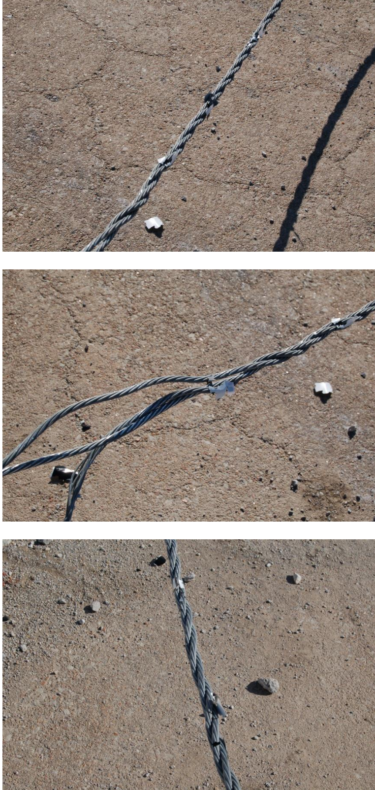
Figure 133. Wire Rope Damage, Test No. DBC-4
