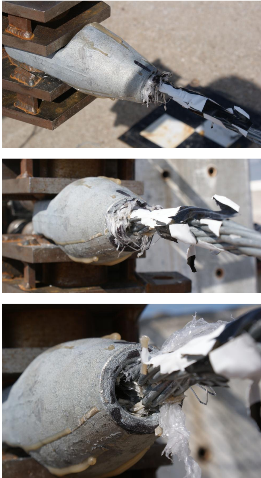
Figure 56. Upstream Wire Rope Damage at Socket, Test No. DTC-1
