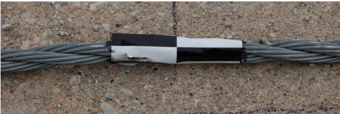
Figure 143. Wire Rope Damage, Test No. DBC-5
