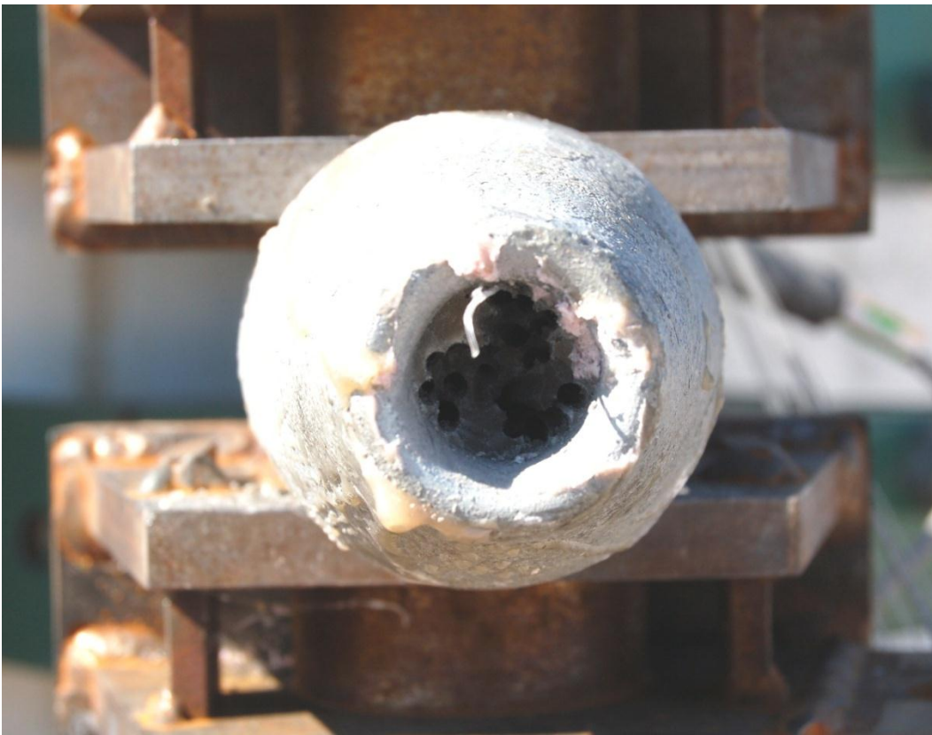
Figure 129. Wire Rope Pullout Through Epoxy, Test No. DBC-3
