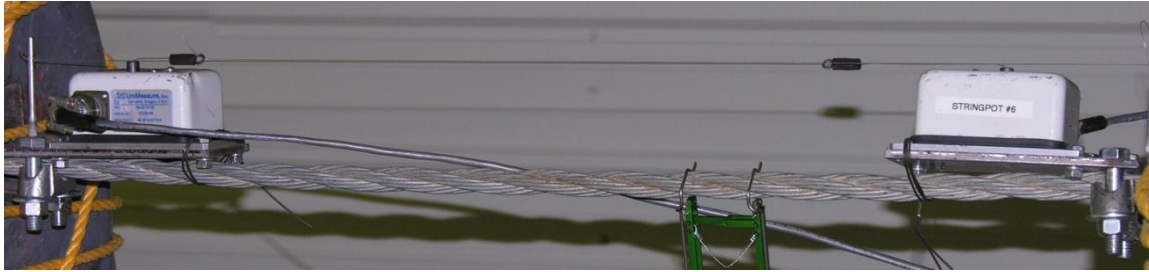
Figure 8. String Pot Setup and Gauge Length
